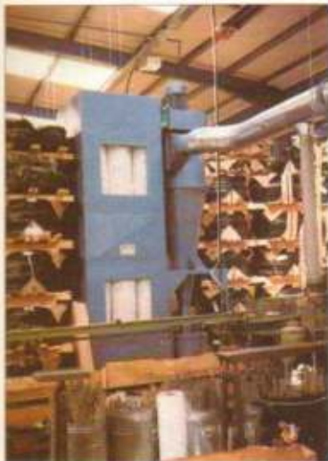
• Model 750 powered Turbaway cyclone with enclosed after filter on aluminium cut off saws application.
