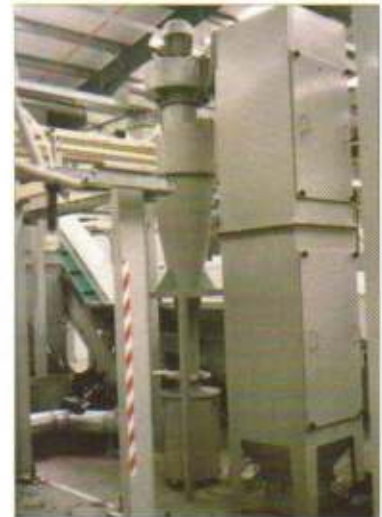
• Model 600 powered Turbaway with enclosed hand shake after filter. Robot plastic cutter.
