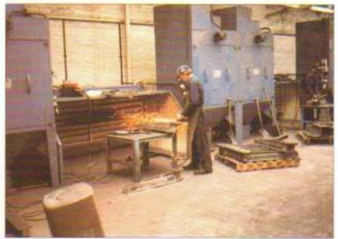
● 9' 0" wide low profile fettling booth with two model FWB500 Dustaway auto shake dust collectors in foundry.
