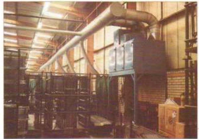
• Centralised welding fume extract system with Smokaway model FF10200. Re-circulation of clean air.
