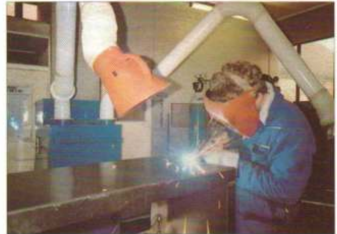
• Fume extraction from welding operation using 3 metre long extract arm on a Smokaway model FF1700
