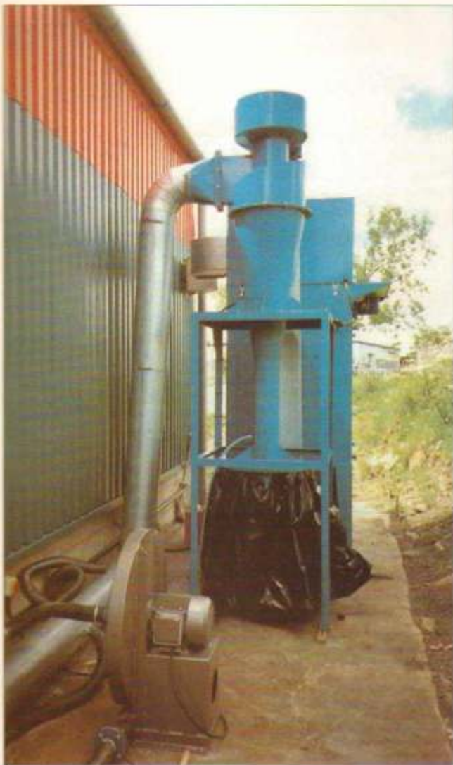
• Model 500 unpowered Turbaway cyclone and Dustaway model FUB375 with hand tool high pressure fan.
