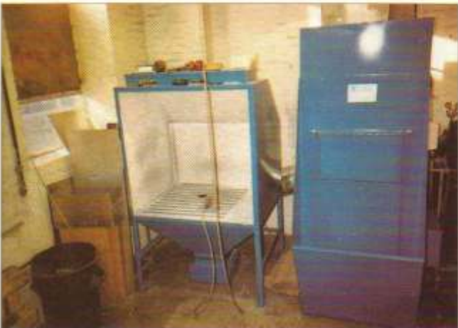
● 4'0" Wide downdraft work bench with model W2000 self induced wet dust collector.
