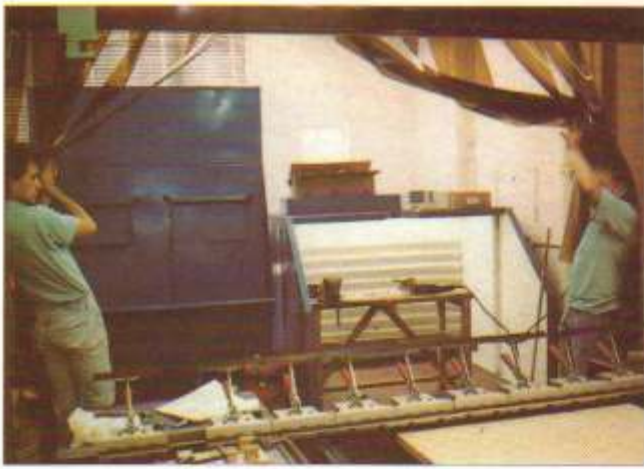
● 6'0" wide low profile fettling booth and model W4000 self induced wet dust collector.
