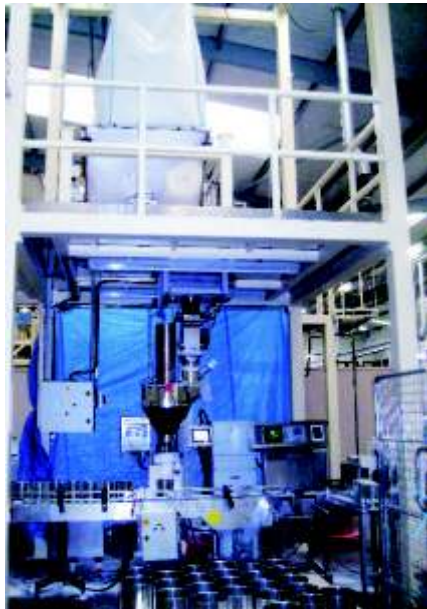
Food industry standard stainless steel hoppers filling points and breeches pieces.
