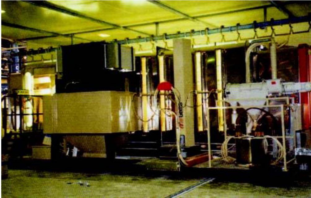
Automatic/manual powder coating booth 9 metres long in stainless steel with three model Cf20 integral cartridge recovery units on Ro/Ro plinth.
