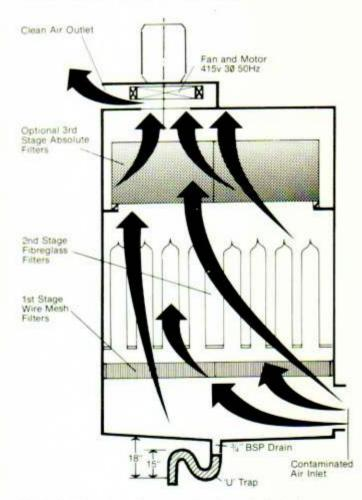
With the fan turned on, contaminated air is drawn through the inlet into the cabinet and past the washable wire mesh 1st stage filters, which separate out chips and large droplets. Fine particles and droplets are captured in the high-efficiency fibreglass 2nd stage filters, and clean air is exhausted from the fan housing outlet. Moisture collected in the filters drains to the bottom of the
